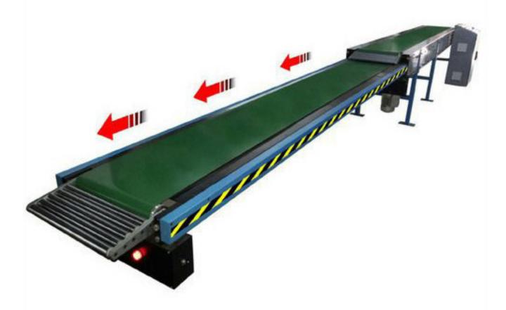
These Conveyors can be installed either on a loading dock or on ground level where a high-level chassis and inclined tail conveyor are included.
